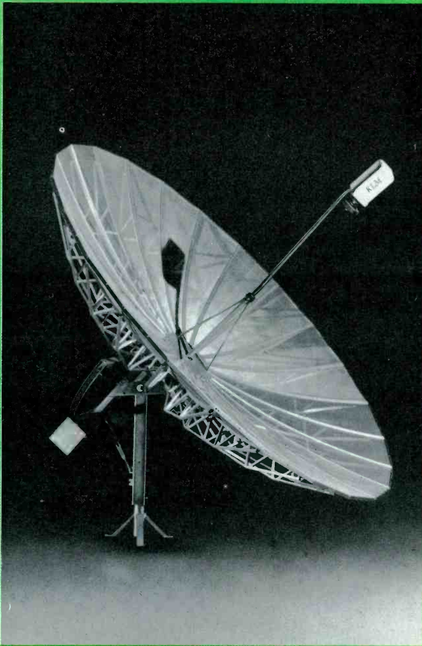
Figure 2. The TVRO dish is a reflector that focuses signals received over a large area onto the opening of a small section of waveguide. The antenna is a probe about 1-inch long mounted at the end of the waveguide.
